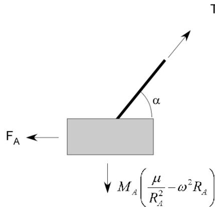
Figure 3. Boundary Conditions at Point A
